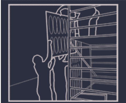
11. Remove the third module. For this operation, you will need a double-flight scaffolding.
